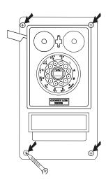
For additional stability, you can also use the supplied rubber spacers in addition to the screws. After you insert the screws through the phone's mounting holes, place a rubber spacer over each screw, so the spacer is between the back of the phone and the wall, then place the phone against the wall
